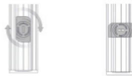
Unlocked Position: rotate clockwise to lock Locked Position
